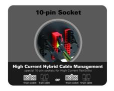
There are two 5-pin black jacks and four 10-pin red jacks on the back of your HCG-520M PSU. These jacks are for the optional cables that come with your power supply. A modular 10-pin connector system allows you plug 5-pin connectors into the 10-pin jacks if you run out of 5-pin jacks.
